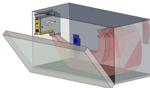
We recommend that the ToolBox Heater be mounted in the upper part of the toolbox.
